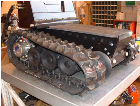
Fig 5-33 Typical displaced track
