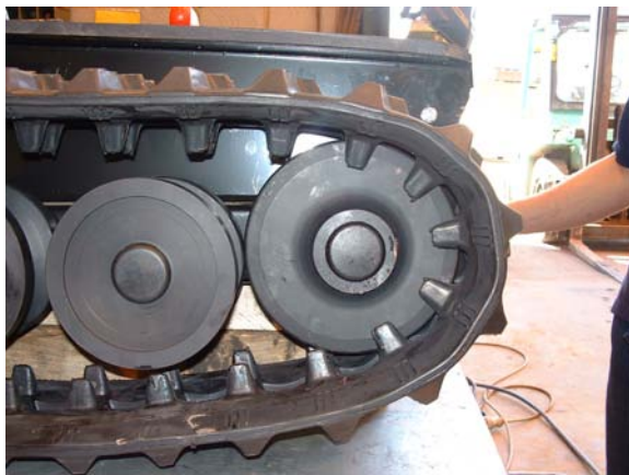
Fig 5-46 Blanking plug fitted
