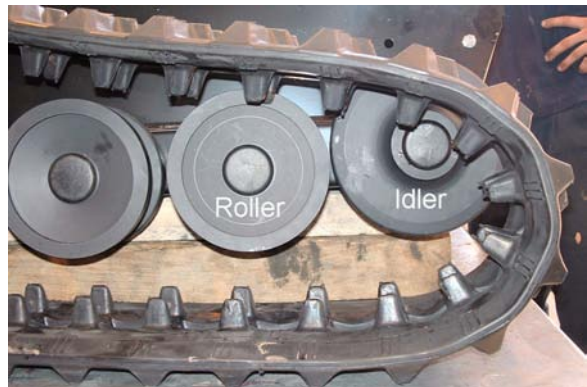
Fig 5-38 Idler touching roller
