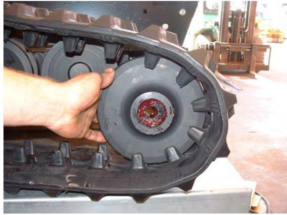
Fig 5-42 Idler in drive track
