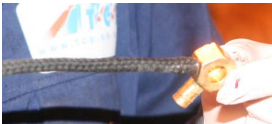
Fig 5-14 Fuel vent tubing
