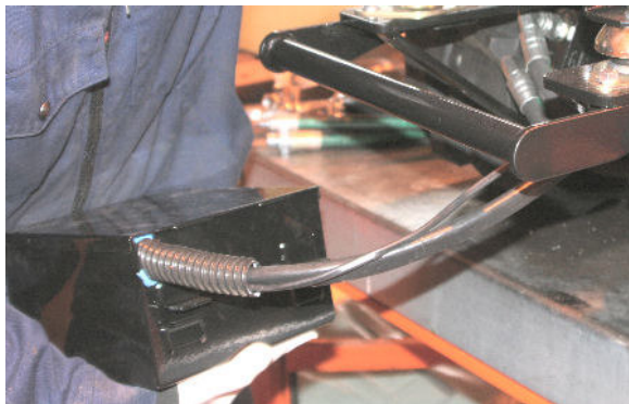
Fig 5-14 Battery box removed
