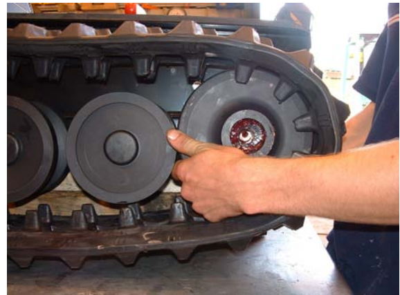
Fig 5-43 Idler on shaft
