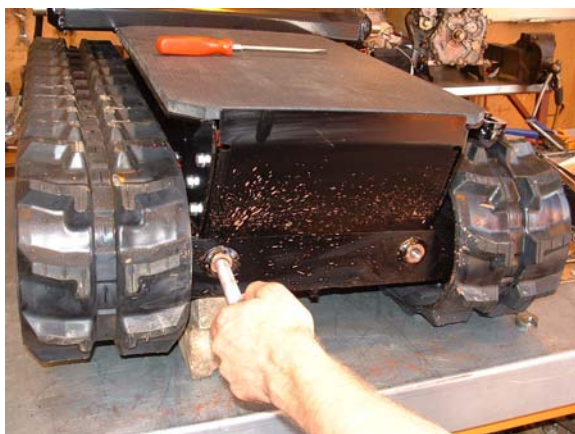
Fig 5-47 Jacking bolts removed
