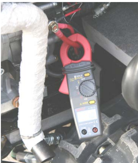
Fig 4-2 Starter current check
