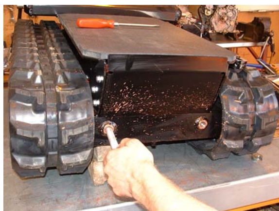
Fig 5-47 Jacking bolts removed
