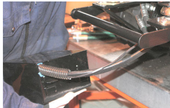
Fig 5-13 Battery box removed
