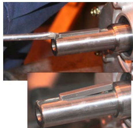
Fig 5-8 Removing shaft key
