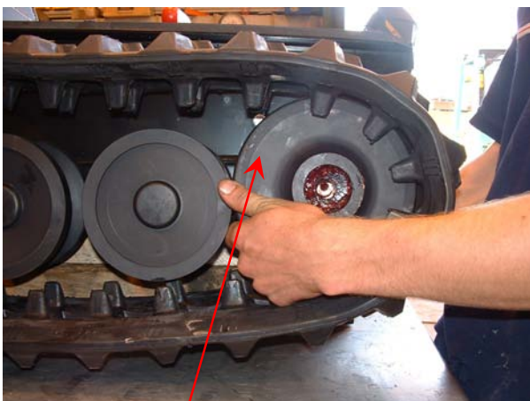
Slide drive track and Idler on shaft
