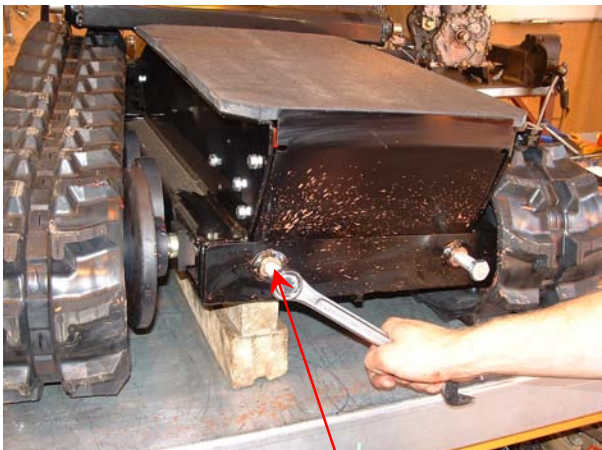
Insert jacking bolts adjust equally
