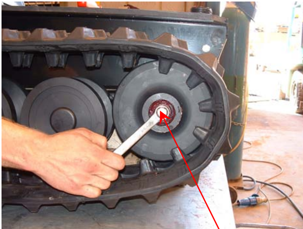
Install securing bolt (torque 49Nm)
