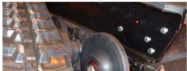
Adjust until idler is in line with roller
