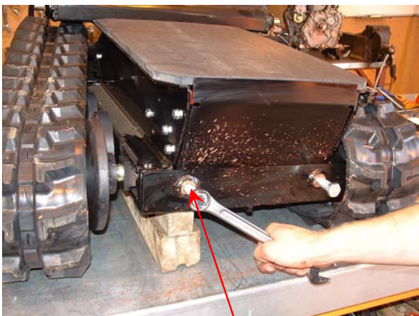
Insert jacking bolts adjust equally
