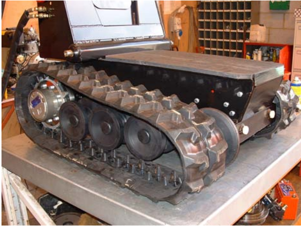
Typical view of displaced track
