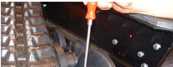
Insert jacking bolts adjust equally
