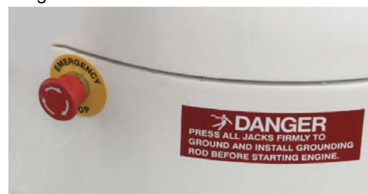
Fig 2-18 Emergency Stop button
