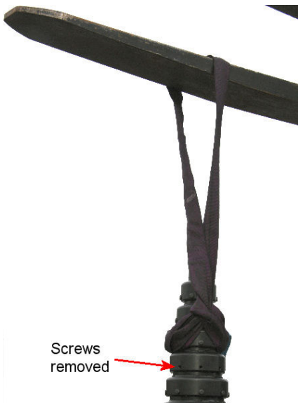
Fig 5-24 Hoisting mast section
