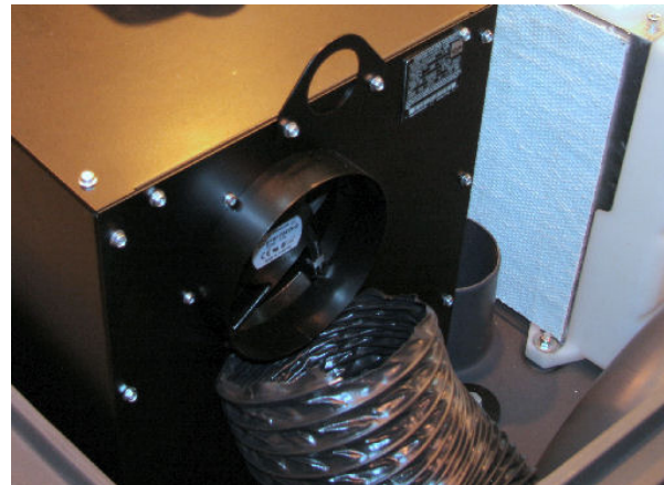
Fig 5-15 Engine extractor duct
