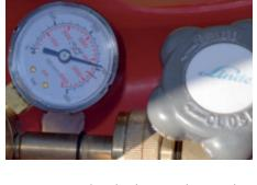
Turn pressure adjust knob on regulator until output gauge shows 4 barg (minimum for BOC's HYMERA® fuel cell).
