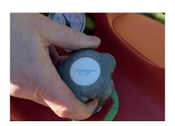
Slowly open the valve on the top of the GENIE® hydrogen cylinder until it is fully open and then turn back half a turn. Check that the contents gauge on regulator shows approximately 300 bar (for a full cylinder).
