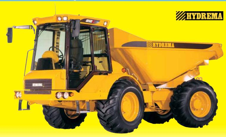
Introducing the Hydrema 912C Multi-tip Dumptruck available for hire from TCP This versatile dumptruck with a 10 tonne load capability is fitted with low ground pressure tyres, designed to get the job done over a variety of terrains in an economic and efficient manner. Constant 4WD is transmitted through a powershift transmission with torque converter, from the powerful turbo diesel engine.
