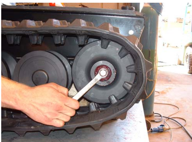
Slide drive track and Idler on shaft
