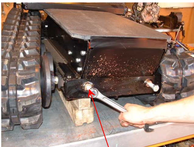
Insert jacking bolts adjust equally
