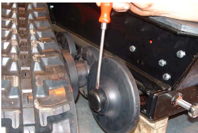
Insert jacking bolts adjust equally
